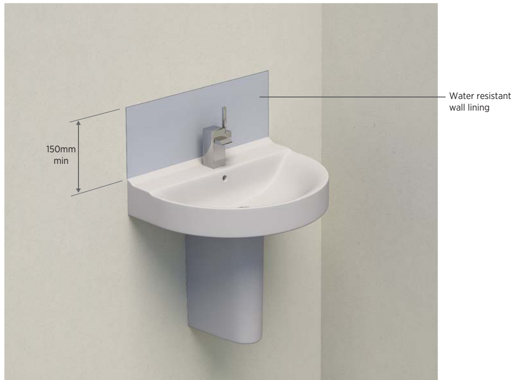
Figure 58: Waterproofing of basin
