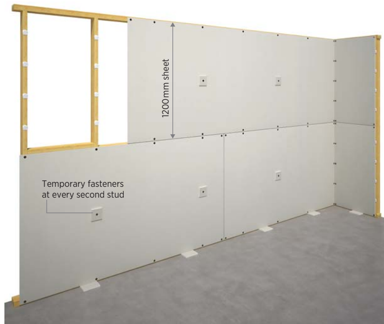
Figure 30: Combination adhesive and screw fixing on walls
