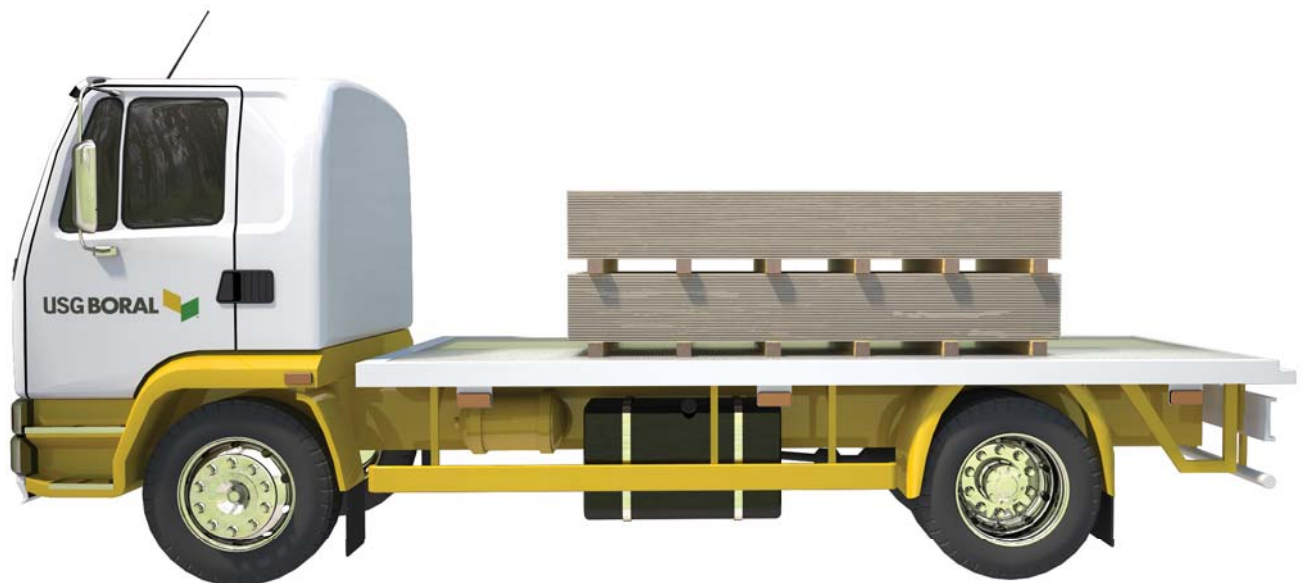
Figure 12: How to position a load
