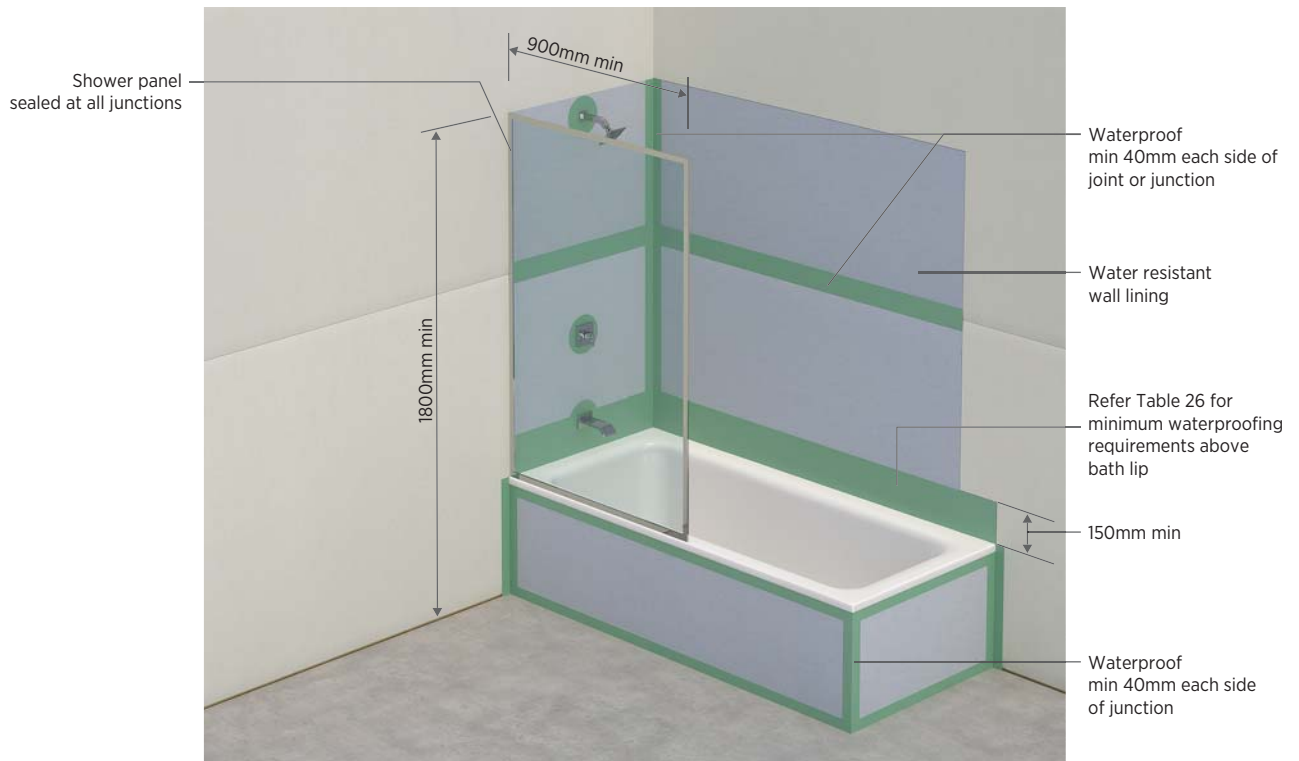
Figure 53: Waterproofing of enclosed shower over bath
